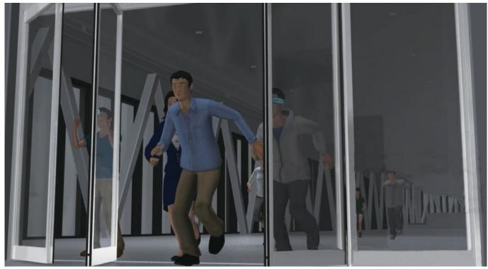
In case of dangerous circumstances such as a fire or power outage due to earthquake, the door can be opened 90 degrees outwards singlehandedly to facilitate escape.
